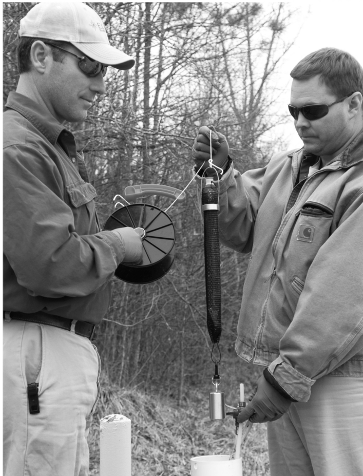
Fig. 4.39. Groundwater sampling at Y-12. Technicians use a passive diffusion bag to sample for volatile organic compounds in groundwater.
